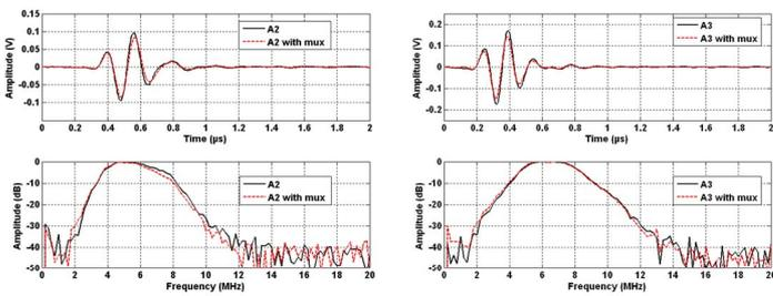
Figure 3 : Time response, frequency response of A2 (left) and A3 (right) central elements with and without multiplexing electronics at the focal distance in water on flat steel target.
