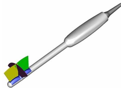
Figure 1 : Illustration showing probe and scan planes provided by the 3 arrays
