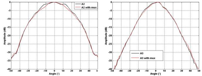
Figure 4 : Directivity pattern at focal point of A2 (left) and A3 (right) array without (solid line) and with (dashed line) ICs in the handle
