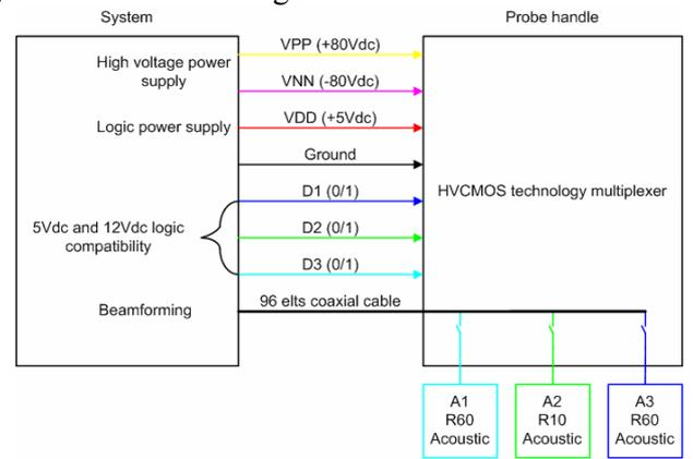
Figure 2 : Block diagram of multiplexing electronic and system front-end requirements
