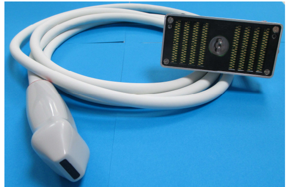
Fig. 3 : Photograph of the complete 128 elements array
