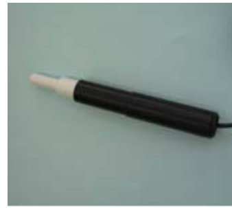
Figure 4 : Photo of single element transducer integrating autoclavable compatible technology.
