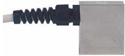
Figure 1 : Photo of the final array packaged and interconnect for harsh environment.
