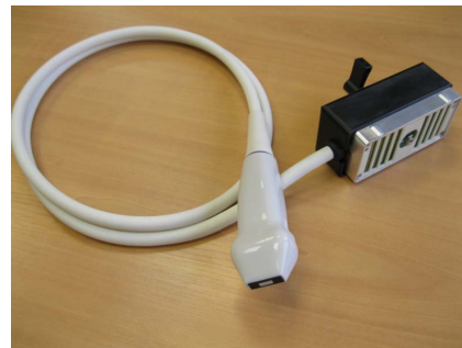
Figure 2 : Photography of the complete 128 elements array
